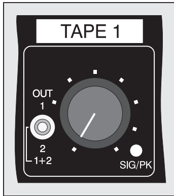
Figure 11. Detail of front panel showing installation-specific labeling
