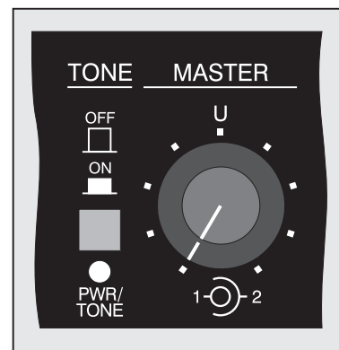
Figure 16. Detail of front panel showing reference tone on/off button and reference tone active LED
